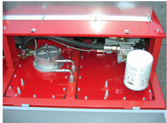
Back view of the machine with the air filter and the water refrigerator connections.
